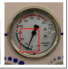
Troubleshooting: If you cannot achieve the desired pressures, try changing the liters on the flow meter or turning the Max Pressure Relief knob located under the flap.
