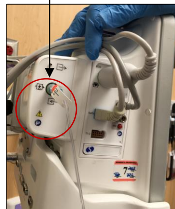
Plug into cartridge on back of monitor.
